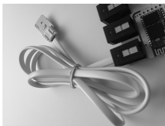
Fig. 2. BITalino or third party sensors can be connected by cable to the main board in any user-defined configuration.
